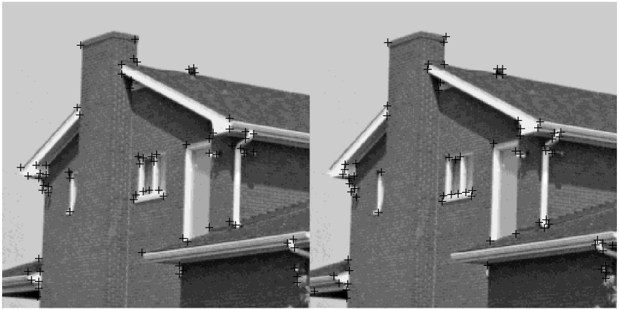
Fig. 3. Left: first 75 corner features detected with the Harris detector and subsequent non-maximum suppression. Right: first 75 corner features detected with the proposed combination of energy tensor and channel clustering.
