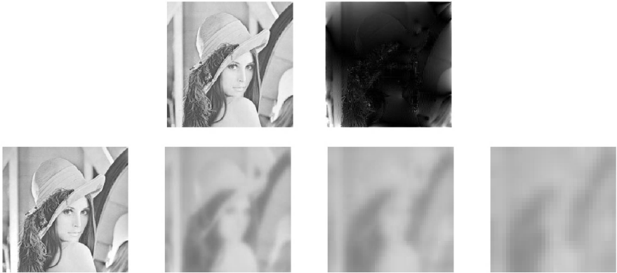
Fig. 3. Image reconstruction in the monogenic scale space. The original image and the absolute error image multiplied by 8 are shown in the top row. Bottom row: right three images demonstrate the intermediate reconstruction in the monogenic scale space, the left image indicates the final result.
