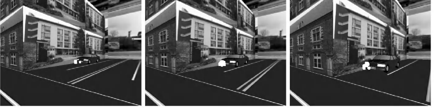
Fig. 4. Some images from the synthetic intersection sequence. The camera is moving on a straight line, while the car in the image is on a collision course. Points where the filter output is above a threshold of 0.35 are marked white.
