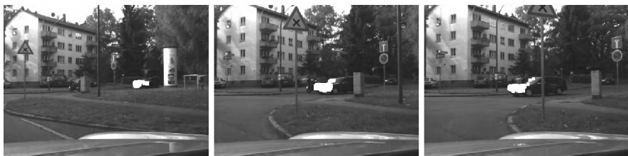
Fig. 5. Some images from a real intersection sequence. Points where the spatio-temporal filter output is above 0.35 are marked white.
