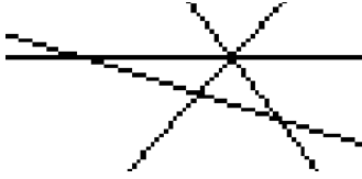
Fig. 1. Line junctions drawn on a grid usually occupy more than a single pixel and have rather unpredictable shapes. This can only be prevented with a real-valued (vector) representation.
